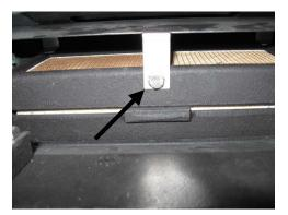
4. Remove the catalytic combustor from the stove. If you have not already done so remove the transport bolts with a <sup>1</sup>/<sub>2</sub>" wrench. The bolts do not need to be returned to the stove. Turn the combustor 90 degrees to remove it. Remove the gasket from around the combustor opening in the combustor pan. Use a putty knife and wire brush to remove any residual gasket or glue. Vacuum up any loose debris.
